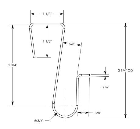
CHANNELS ARE NOTCHED FOR GROUND CABLE CLIPS.
