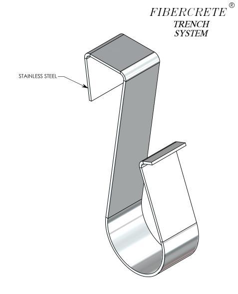
CHANNELS ARE NOTCHED FOR GROUND CABLE CLIPS.
