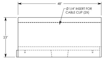
**NOTE 1:** FOR NON-STANDARD LENGTHS THE CHANNEL WILL BE SOLID BOTTOM AND DESIGNATED WITH ITS CORRESPONDING LENGTH MEASUREMENT. IE: 801016HT3 32"
