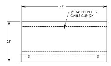
**NOTE 1:** FOR NON-STANDARD LENGTHS THE CHANNEL WILL BE DESIGNATED WITH ITS CORRESPONDING LENGTH MEASUREMENT. IE: 801016HT3 32"
