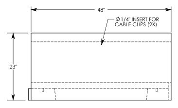
NOTE: FOR NON-STANDARD LENGTHS THE CHANNEL WILL BE SOLID BOTTOM AND DESIGNATED WITH ITS CORRESPONDING LENGTH MEASUREMENT. IE: 801016LT 32"
