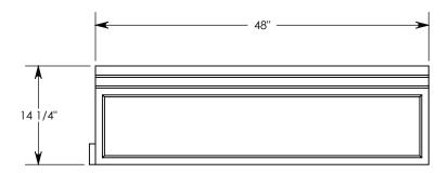
NOTE: FOR NON-STANDARD LENGTHS THE CHANNEL WILL BE SOLID BOTTOM AND DESIGNATED WITH ITS CORRESPONDING LENGTH MEASUREMENT. IE: 8010F 32"
