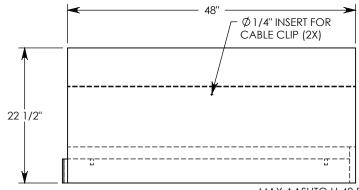
**NOTE 1:** FOR NON-STANDARD LENGTHS THE CHANNEL WILL BE SOLID BOTTOM AND DESIGNATED WITH ITS CORRESPONDING LENGTH MEASUREMENT. IE: 8010HT 32"
