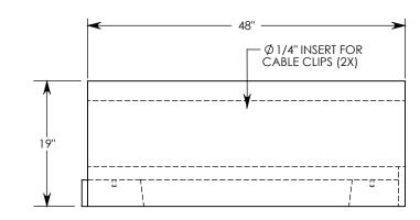
NOTE: FOR NON-STANDARD LENGTHS THE CHANNEL WILL BE SOLID BOTTOM AND DESIGNATED WITH ITS CORRESPONDING LENGTH MEASUREMENT. IE: 8010LT 32"
