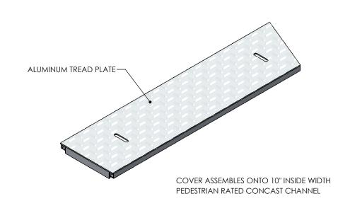
NOTE 1: FOR NON-STANDARD LENGTHS THE PART NUMBER WILL CORRESPOND TO IT'S MEASURED LENGTH. IE: 8011AT 22.5R 24"
