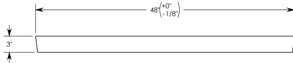
**NOTE 1:** FOR NON-STANDARD LENGTHS THE CHANNEL WILL BE SOLID BOTTOM AND DESIGNATED WITH ITS CORRESPONDING LENGTH MEASUREMENT. IE: 8011HT3P 16"
