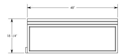
NOTE: FOR NON-STANDARD LENGTHS THE CHANNEL WILL BE DESIGNATED WITH ITS CORRESPONDING LENGTH MEASUREMENT. IE: 802016FSB 32"
