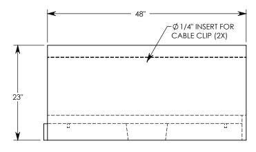
**NOTE 1:** FOR NON-STANDARD LENGTHS THE CHANNEL WILL BE SOLID BOTTOM AND DESIGNATED WITH ITS CORRESPONDING LENGTH MEASUREMENT. IE: 802016HT3 32"
