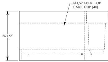
MAX AASHTO H-40 RATED - 64,000 LB. SINGLE AXLE LOAD DEPENDENT ON TRENCH COVER RATING MINIMUM ALLOWABLE SOIL BEARING PRESSURE – H-40: 3,500 PSF; H-20: 3,000 PSF
