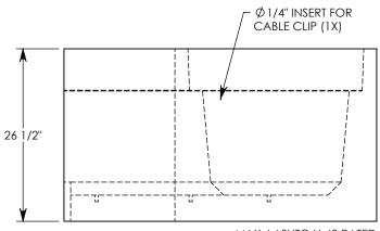
MAX AASHTO H-40 RATED - 64,000 LB. SINGLE AXLE LOAD DEPENDENT ON TRENCH COVER RATING MINIMUM ALLOWABLE SOIL BEARING PRESSURE – H-40: 4,000 PSF; H-20: 3,000 PSF
