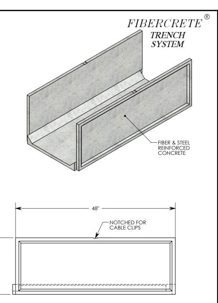
NOTE: FOR NON-STANDARD LENGTHS THE CHANNEL WILL BE DESIGNATED WITH ITS CORRESPONDING LENGTH MEASUREMENT. IE: 802016SB 32"
