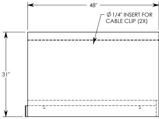
**NOTE 1:** FOR NON-STANDARD LENGTHS THE CHANNEL WILL BE SOLID BOTTOM AND DESIGNATED WITH ITS CORRESPONDING LENGTH MEASUREMENT. IE: 802024HT3 32"
