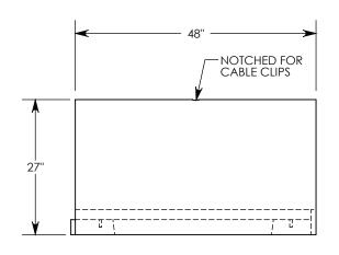
**NOTE:** FOR NON-STANDARD LENGTHS THE CHANNEL WILL BE SOLID BOTTOM AND DESIGNATED WITH ITS CORRESPONDING LENGTH MEASUREMENT. IE: 802024PT 32"
