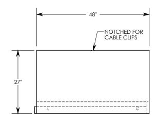
**NOTE:** FOR NON-STANDARD LENGTHS THE CHANNEL WILL BE SOLID BOTTOM AND DESIGNATED WITH ITS CORRESPONDING LENGTH MEASUREMENT. IE: 802024PTSB 32"
