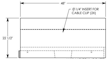
**NOTE 1:** FOR NON-STANDARD LENGTHS THE CHANNEL WILL BE SOLID BOTTOM AND DESIGNATED WITH ITS CORRESPONDING LENGTH MEASUREMENT. IE: 8020HT 32"
