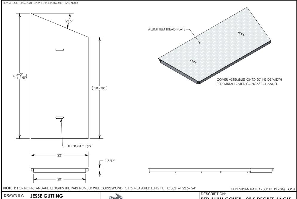
CREATED DATE: 3/22/2010 REVISION LEVEL: A 4/27/2020 SAVED DATE: SAVED BY: jgutting WEIGHT: MATERIAL: **WELDED ALUMINUM** 26 LBS.
