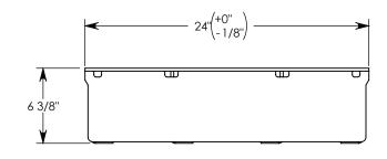
NOTE 1: FOR NON-STANDARD LENGTHS THE PART NUMBER WILL CORRESPOND TO IT'S MEASURED LENGTH. IE: 8021HTSG40 16" NOTE 2: TREAD ON DIAMOND PLATE ADDS 1/8" TO OVERALL HEIGHT
