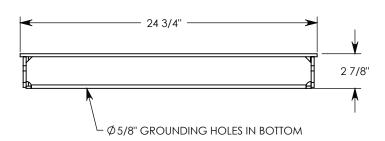
NOTE 1: FOR NON-STANDARD LENGTHS, THE PART NUMBER WILL CORRESPOND TO IT'S MEASURED LENGTH. IE: 8021HTSG 22.5L 18" NOTE 2: TREAD ON DIAMOND PLATE ADDS 1/8" TO THE OVERALL HEIGHT
