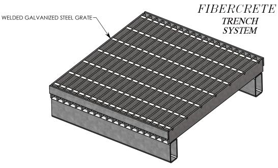
COVER ASSEMBLES ONTO 20" INSIDE WIDTH HEAVY TRAFFIC H-20 RATED CONCAST CHANNEL.
