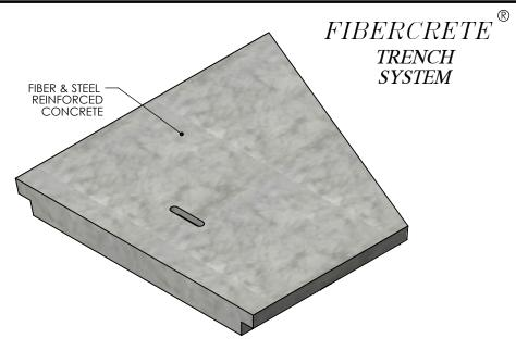
COVER ASSEMBLES ONTO 20" INSIDE WIDTH PEDESTRIAN RATED CONCAST CHANNEL.
