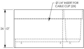
MAX AASHTO H-40 RATED - 64,000 LB. SINGLE AXLE LOAD DEPENDENT ON TRENCH COVER RATING MINIMUM ALLOWABLE SOIL BEARING PRESSURE – H-40: 3,000 PSF; H-20: 3,000 PSF
