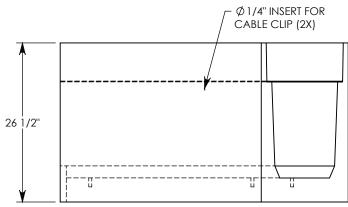
MAX AASHTO H-40 RATED - 64,000 LB. SINGLE AXLE LOAD DEPENDENT ON TRENCH COVER RATING
