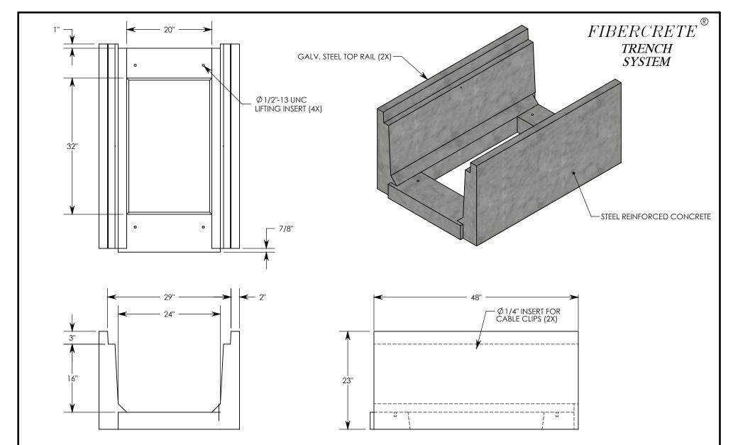
NOTE: FOR NON-STANDARD LENGTHS THE CHANNEL WILL BE SOLID BOTTOM AND DESIGNATED WITH ITS CORRESPONDING LENGTH MEASUREMENT. IE: 802416LT 32"
