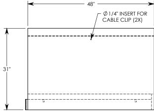
**NOTE 1:** FOR NON-STANDARD LENGTHS THE CHANNEL WILL BE SOLID BOTTOM AND DESIGNATED WITH ITS CORRESPONDING LENGTH MEASUREMENT. IE: 802424HT3 32"
