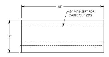
**NOTE 1:** FOR NON-STANDARD LENGTHS THE CHANNEL WILL BE SOLID BOTTOM AND DESIGNATED WITH ITS CORRESPONDING LENGTH MEASUREMENT. IE: 8024HT3SB 32"
