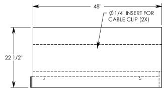
**NOTE 1:** FOR NON-STANDARD LENGTHS THE CHANNEL WILL BE SOLID BOTTOM AND DESIGNATED WITH ITS CORRESPONDING LENGTH MEASUREMENT. IE: 8024HT 32"
