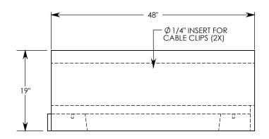
NOTE: FOR NON-STANDARD LENGTHS THE CHANNEL WILL BE SOLID BOTTOM AND DESIGNATED WITH ITS CORRESPONDING LENGTH MEASUREMENT. IE: 8024LT 32"
