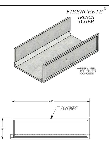
NOTE: FOR NON-STANDARD LENGTHS THE CHANNEL WILL BE DESIGNATED WITH ITS CORRESPONDING LENGTH MEASUREMENT. IE: 8024SB 32"
