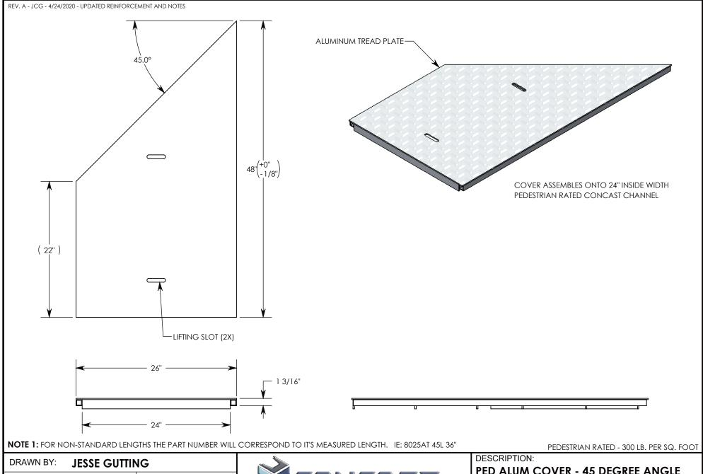
CREATED DATE: 3/22/2010 REVISION LEVEL: A 4/27/2020 SAVED DATE: SAVED BY: jgutting WEIGHT: MATERIAL: **WELDED ALUMINUM** 25 LBS.
