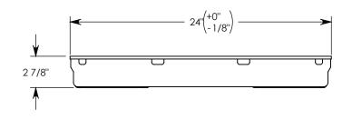
**NOTE 1:** FOR NON-STANDARD LENGTHS THE PART NUMBER WILL CORRESPOND TO IT'S MEASURED LENGTH. IE: 8025HTSG 16" **NOTE 2:** TREAD ON DIAMOND PLATE ADDS 1/8" TO OVERALL HEIGHT
