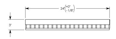
NOTE 1: FOR NON-STANDARD LENGTHS, THE PART NUMBER WILL CORRESPOND TO IT'S MEASURED LENGTH. IE:8025HTSGV 18"
