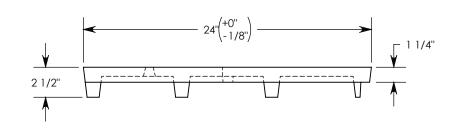
**NOTE 1:** FOR NON-STANDARD LENGTHS, THE PART NUMBER WILL CORRESPOND TO IT'S MEASURED LENGTH. IE: 8025PTP 22.5L 18"
