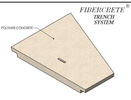
COVER ASSEMBLES ONTO 24" INSIDE WIDTH PEDESTRIAN RATED **PT** CONCAST CHANNEL.
