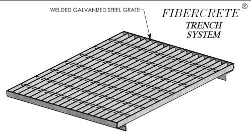
COVER ASSEMBLES ONTO 24" INSIDE WIDTH PEDESTRIAN RATED CONCAST PT CHANNEL.
