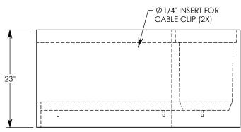
MAX AASHTO H-40 RATED - 64,000 LB. SINGLE AXLE LOAD DEPENDENT ON TRENCH COVER RATING MINIMUM ALLOWABLE SOIL BEARING PRESSURE – H-40: 3,000 PSF; H-20: 3,000 PSF
