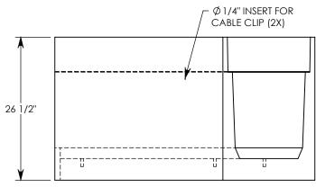
MAX AASHTO H-40 RATED - 64,000 LB. SINGLE AXLE LOAD DEPENDENT ON TRENCH COVER RATING MINIMUM ALLOWABLE SOIL BEARING PRESSURE – H-40: 3,000 PSF; H-20: 3,000 PSF
