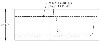
MAX AASHTO H-40 RATED - 64,000 LB. SINGLE AXLE LOAD DEPENDENT ON TRENCH COVER RATING MINIMUM ALLOWABLE SOIL BEARING PRESSURE – H-40: 3,000 PSF; H-20: 3,000 PSF
