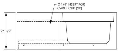
MAX AASHTO H-40 RATED - 64,000 LB. SINGLE AXLE LOAD DEPENDENT ON TRENCH COVER RATING
