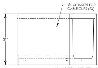
MAX AASHTO H-40 RATED - 64,000 LB. SINGLE AXLE LOAD DEPENDENT ON TRENCH COVER RATING
