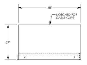
**NOTE:** FOR NON-STANDARD LENGTHS THE CHANNEL WILL BE SOLID BOTTOM AND DESIGNATED WITH ITS CORRESPONDING LENGTH MEASUREMENT. IE: 803024PTSB 32"
