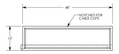
NOTE: FOR NON-STANDARD LENGTHS THE CHANNEL WILL BE DESIGNATED WITH ITS CORRESPONDING LENGTH MEASUREMENT. IE: 8030SB 32"
