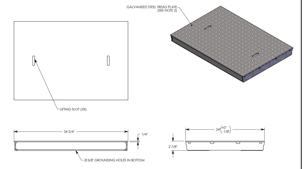
**NOTE 1:** FOR NON-STANDARD LENGTHS, THE PART NUMBER WILL CORRESPOND TO IT'S MEASURED LENGTH. IE: 8031HTSG 18" **NOTE 2:** TREAD ON DIAMOND PLATE ADDS 1/8" TO OVERALL HEIGHT
