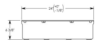
NOTE 1: FOR NON-STANDARD LENGTHS THE PART NUMBER WILL CORRESPOND TO IT'S MEASURED LENGTH. IE: 8031HTSG40 16" NOTE 2: TREAD ON DIAMOND PLATE ADDS 1/8" TO OVERALL HEIGHT
