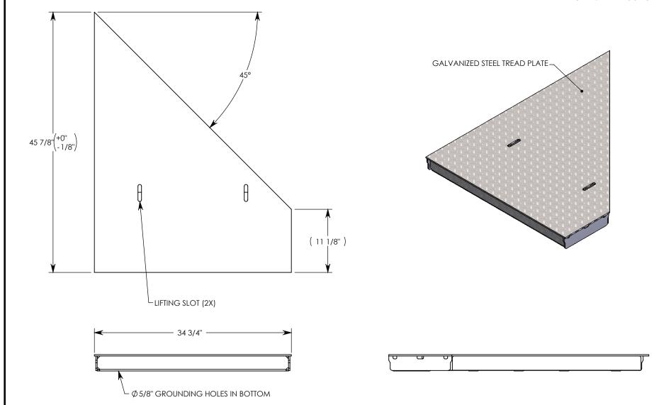
NOTE 1: FOR NON-STANDARD LENGTHS, THE PART NUMBER WILL CORRESPOND TO IT'S MEASURED LENGTH. IE: 8031HTSG 45R 18"
