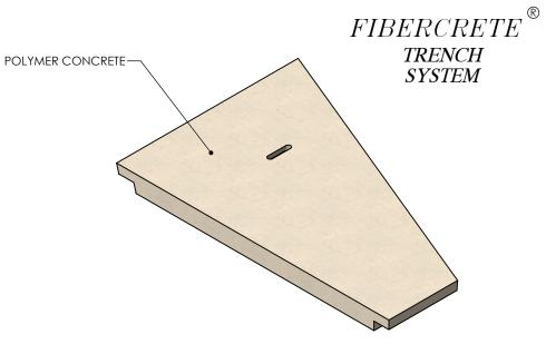
COVER ASSEMBLES ONTO 30" INSIDE WIDTH PEDESTRIAN RATED **PT** CONCAST CHANNEL.
