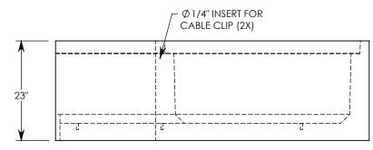
AASHTO H-20 RATED - 32,000 LB, SINGLE AXLE LOAD MINIMUM ALLOWABLE SOIL BEARING PRESSURE – 3,000 PSF
